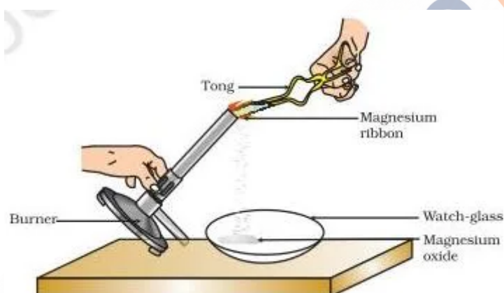
Figure 1.1 Burning of a magnesium ribbon in air and collection of magnesium oxide in a watch-glass. Source: NCERT
