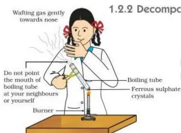
Figure 1.4 Correct way of heating the boiling tube containing crystals of ferrous sulphate and of smelling the odour. Source: NCERT
